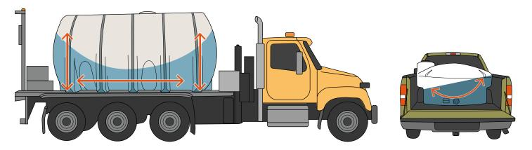
The arrows indicate how the weight of a live load and its centre of gravity can shift. Liquid sloshing around in the tank can have a significant effect on the vehicle's handling and stability.
